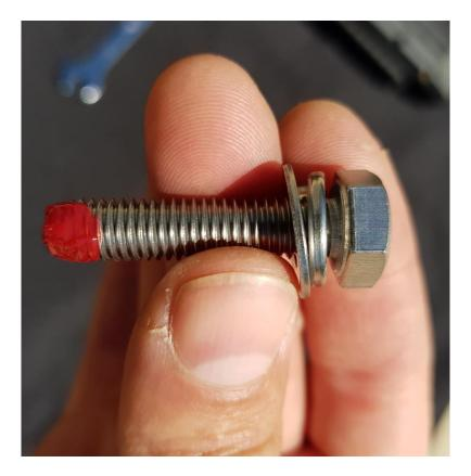
Insert fore-end bolt into the bore of the fore-end, and fit to the front of the chassis action block – Important: Make sure all mating surfaces are clean and free for debris before fitting these parts together. This is critical to alignment of the fore-end assembly.
