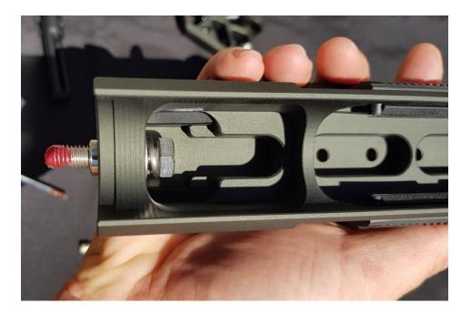
Screw the bolt into the chassis action block with your fingers until you feel resistance of the spring washer. At this stage take your ½" 12-point ring spanner and carefully tighten the bolt, this will need to be tightened firmly, but not overtightened. Important – Be very careful during tightening that bolt, that you do not damage the side rails or finish of the fore-end with the edges of the spanner.
