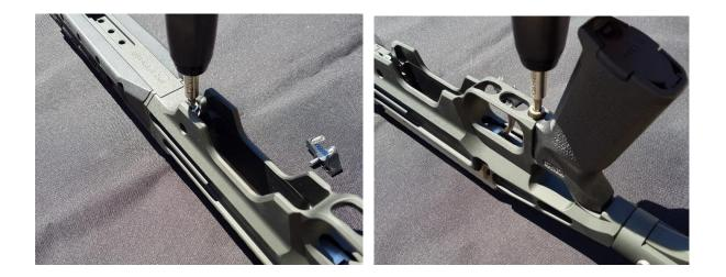
Fitting Magazine Catch – With the spring fitted to the bore of the magazine catch, insert the unit from rear engaging it forward to line up with the retaining pin.
