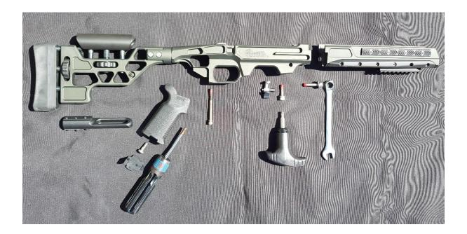
Assemble fore-end bolt, flat washer and spring wash as indicated, ensure the spring washer sits between the head of the bolt and the flat washer (see below)
