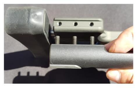
3 – Using a 4mm Allen key tighten screw down firm but not overtight, starting from the centre screw, then the front screw then the rear screw
