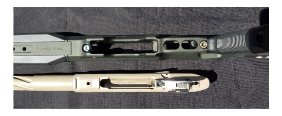
With the barrelled action sitting with the trigger assembly facing upwards, place chassis over the action carefully – Ensure the recoil lug in the stock is keyed into the action slot, the action screws of the action are lined up with corresponding bores in the chassis.
