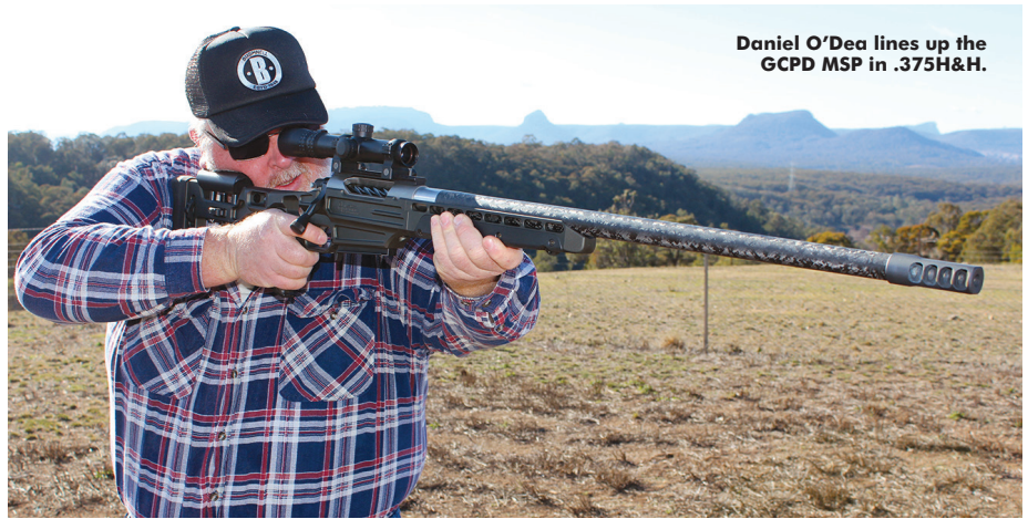
An under barrel style fore-end with composite textured grip panels replaces the more commonly seen tube style fore-end.
