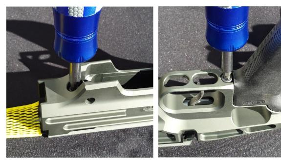
Fitting Magazine Catch – With the spring fitted to the bore of the magazine catch, insert the unit from rear engaging it forward to line up with the retaining pin.
