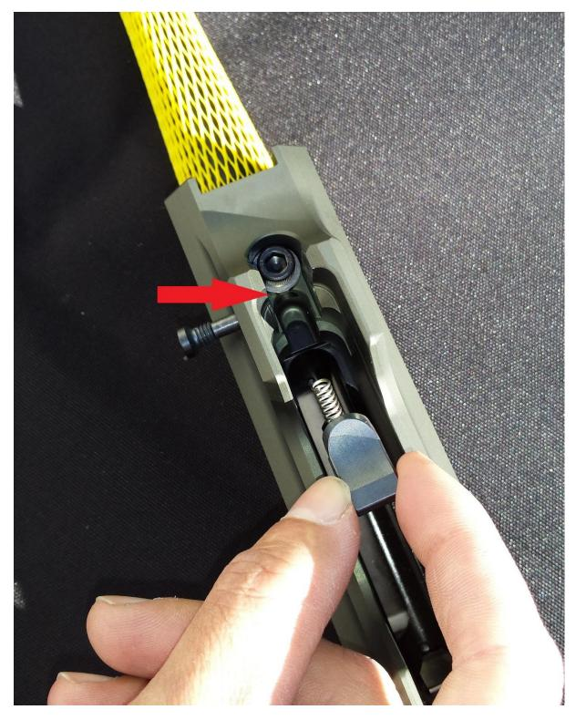
Fitting Fore-End – Check that all mounting faces, tube dowel and corrosponding recess if completely clean and free of debris and the outside of barrel protected.
