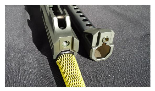
Insert M8 bolt and firmly tighten with 6mm Allen Key.
